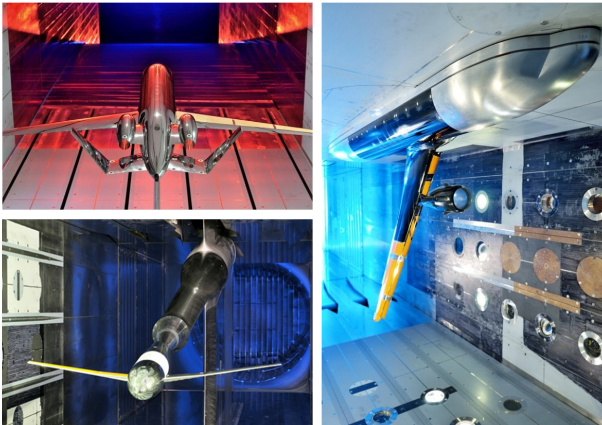
Figure 1: Temperature sensitive paint-coated models in the ETW. Top left: Full model (EC FP7 HiLamBiz). Bottom left: Full model (LuFo V-2 ReSK). Right: Half model (LuFo IV ALSA).
