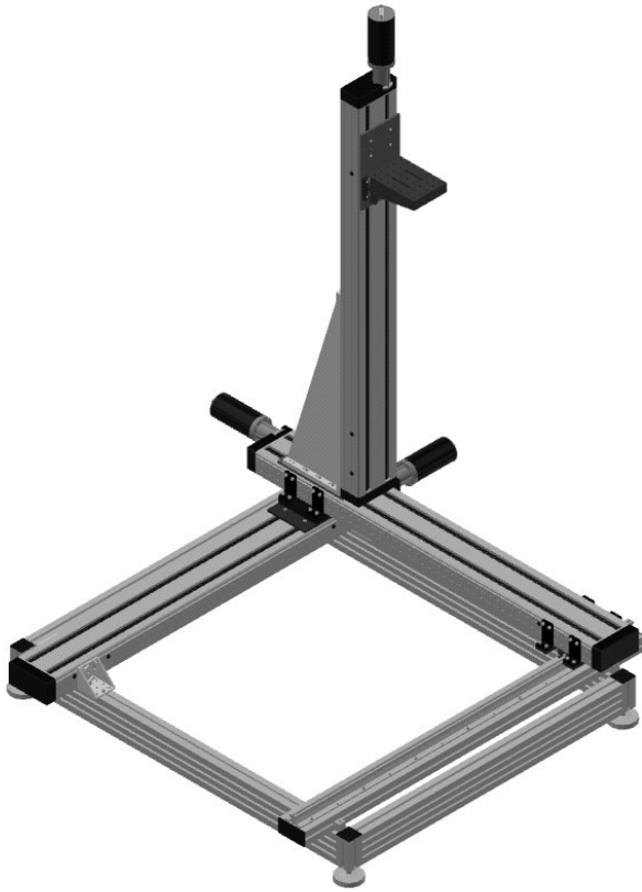
Fig 1: 3D Traversing System with Mounting frame based on isel linear stages and ILA DC-motor modules
