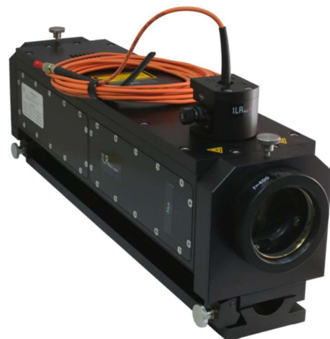
Fig. 2: 2D fp50-shift probe detached from combined probe
