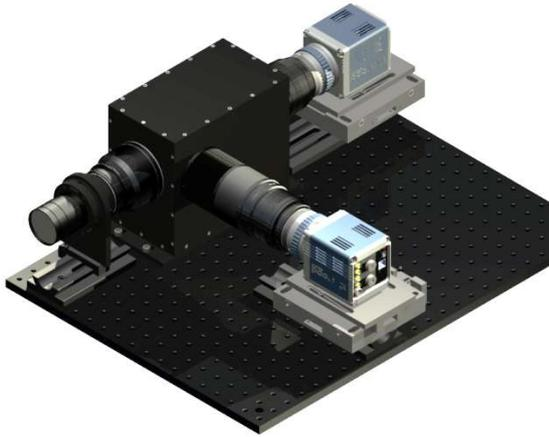
Fig. 1: DGV Camera module (with optics and cameras)
